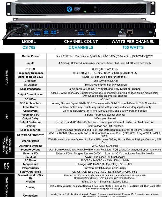
Analog Input: 3 pin Amphenol Anytek, Output: 2 pin Amphenol Anytek, External IO: 3 pin Amphenol Anytek, Connectors Power in: IEC, Ethernet RJ45 In for Control
