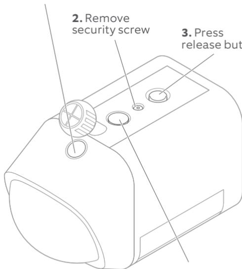
4. Remove weather seal, and insert in unused hole
